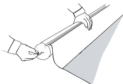
5. Hold cassette and remove guard pin on the left side. The mechanism is now activated.
