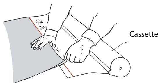
3. Remove protection foil. Position lower end of banner (print upwards) along the red line and affix it.
